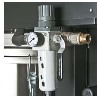
Zariadenie na reguláciu tlaku filtra. Pressure filter regulation device.
